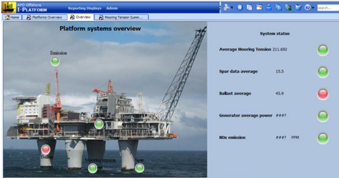
Figure 4: Typical KPI dashboard for subsystems of an offshore oil and gas production platform.
