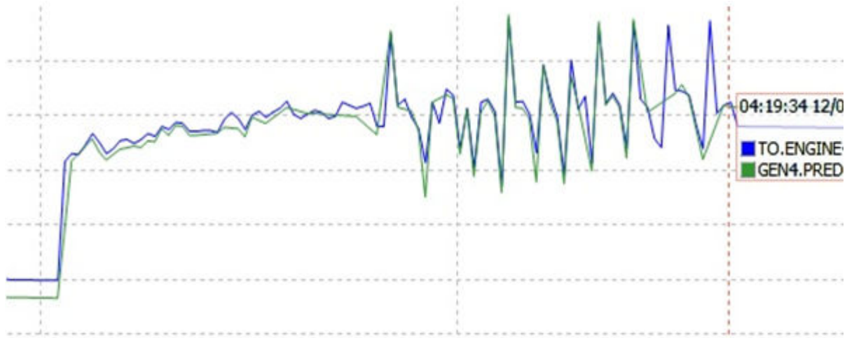
Figure 5: Actual (blue) vs. predicted (green) output for a test data stream from an offshore operating platform.
